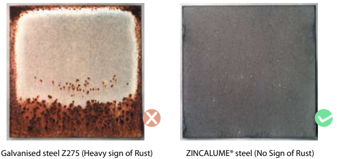
Figure 3: Outdoor Exposure Test and Product Performance after 6 years at severe marine environment
