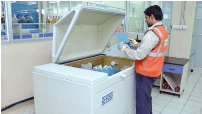
Corrosion Resistance (Q-Fog Salt Spray Tester)
