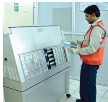
Paint durability (Q-UV Tester)
