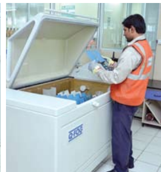
Corrosion Resistance (Q-Fog Salt Spray Tester)
