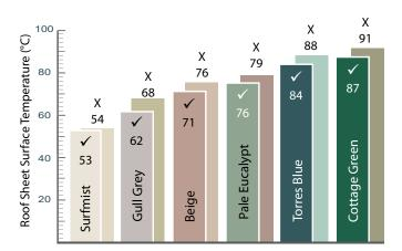
The temperature of the roof sheet is lower due to the THERMATECH™ technology in COLORBOND® steel. This in turn cuts down the heat radiation into the building, making the interior of the building cooler.
