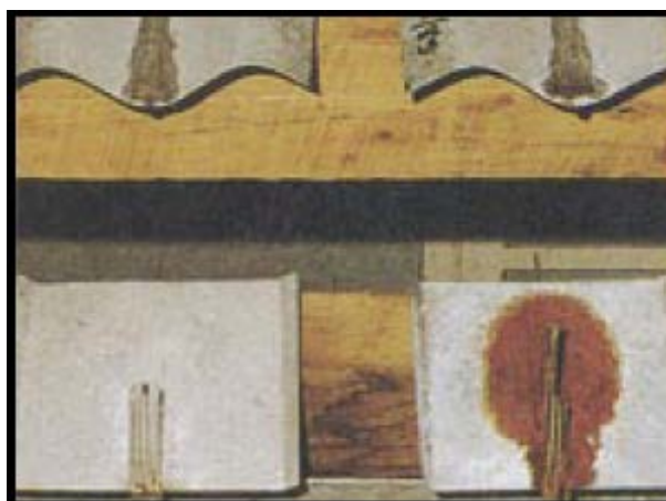
Test 3: ZINCALUME® steel to ZINCALUME® steel gutter (left); ZINCALUME® steel to zinc-coated steel gutter (right).
