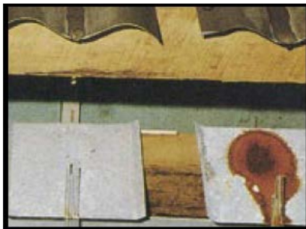
Test 2: COLORBOND® steel to ZINCALUME® steel gutter (left); COLORBOND® steel to zinc-coated steel gutter (right).
