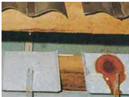
2 COLORBOND® steel to ZINCALUME® steel gutter ( left ) COLORBOND® steel to zinc-coated steel gutter ( right )
