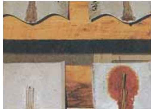
3 ZINCALUME® steel to ZINCALUME® steel gutter ( left ) ZINCALUME® steel to zinc-coated steel gutter ( right )
