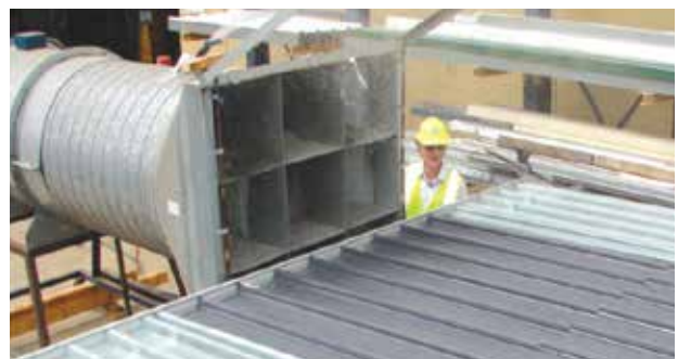
Figure 3: Weather test rig is used to test weather-resistance by blowing simulated wind borne rain.
