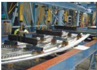
Fig. 2.1 - Formwork - Point Load
