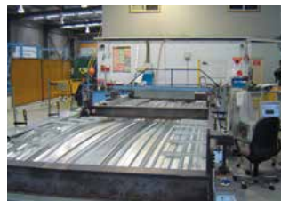
Fig. 2.2 - Formwork - Air Pressure Test
