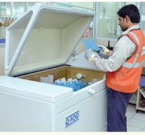
Salt Spray Corrosion Resistance Testing
