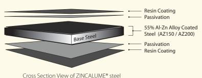
ZINCALUME® steel has 150 g/m² or 200 g/m² metallic coating distributed equally on both surfaces. It is available in Base Metal Thickness (BMT) ranging between 0.30mm to 1.30mm and coil widths of 900 to 1250 mm. It is offered with yield strength of minimum 300 MPa to minimum 550 MPa depending on the application. ZINCALUME® steel
