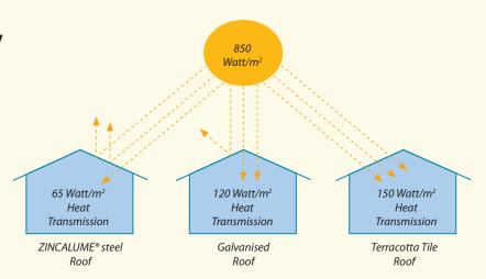
Based on a weather-worn roof where the level of reflectivity had stabilised and which were exposed to solar radiation of 850 W/m<sup>2</sup>
