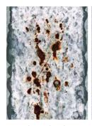
Galvanised steel Z275 @ 240 hours of salt spray testing.
