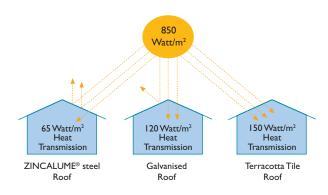
Based on a weather-worn roof where the level of reflectivity had stabilised and which were exposed to solar radiation of  $850\,\mathrm{W/m^2}$
