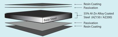
**Cross Section of ZINCALUME® steel**
