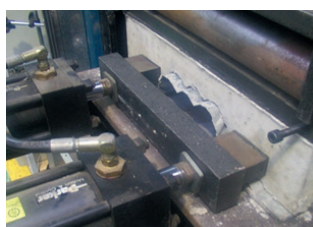
Fig. 2.3 - Composite - Slip Block Test
