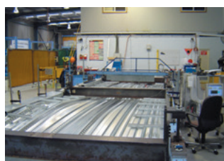
Fig. 2.2 - Formwork - Air Pressure Test
