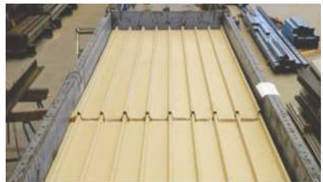
Figure 2: Wind uplift tests were performed to ensure LOK-KLIP™ clips meet the performance standards required.
