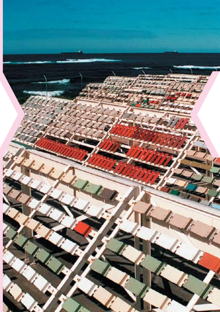
Exposure site : Bellambi Point Australia (Marine)
