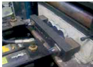
Fig. 2.3 - Composite - Slip Block Test
