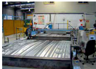
Fig. 2.2 - Formwork - Air Pressure Test
