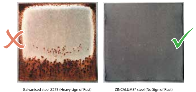
Figure 3: Outdoor Exposure Test and Product Performance after 6 years at severe marine environment
